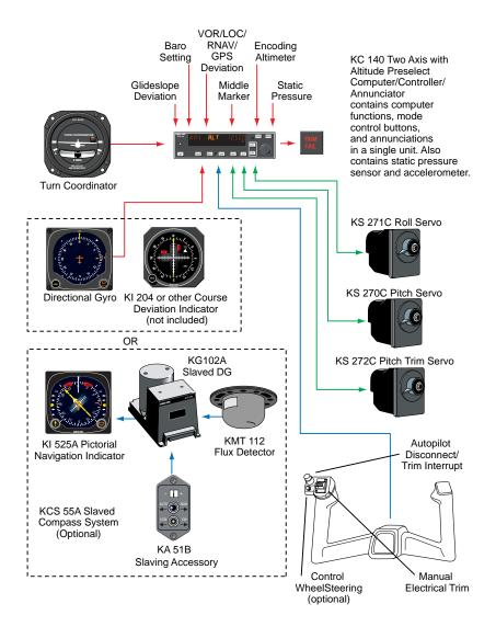
KAP 140 Two Axis/Altitude Preselect System Diagram
