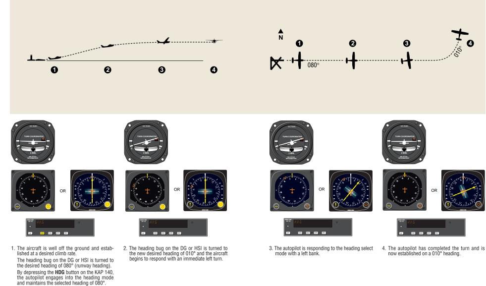
Note: The autopilot controls only the roll axis. The PILOT must maintain control of the pitch and yaw axis.
