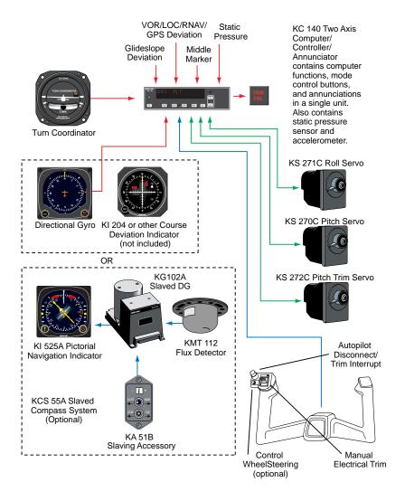
KAP 140 Two Axis System Diagram
